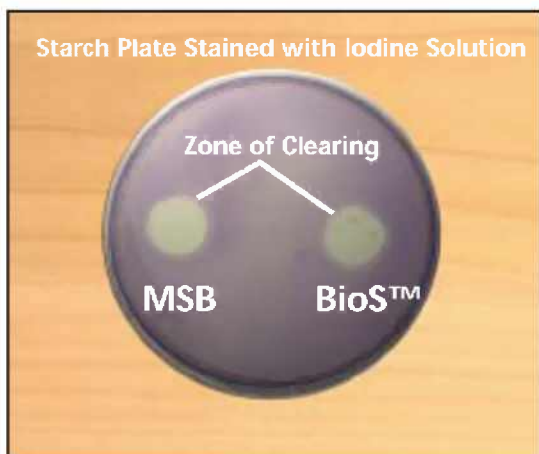
Figure 6. BioS™ and MSB consortiums are each spotted onto separate disks placed on a Petri plate containing a starch medium. As amylase is produced and excreted, the starch is broken down. After the Petri plate is stained with an iodine solution, the zone of clearing becomes visible. As demonstrated, both the BioS™ and MSB consortiums produce considerable levels of amylase.
